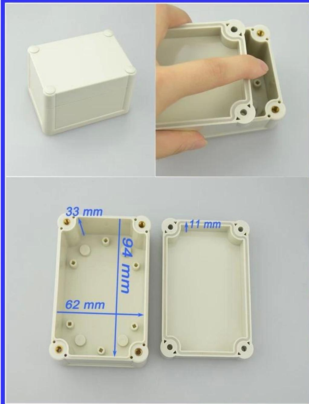
The image displays a white ABS enclosure in three views: a closed perspective, an open view held by a hand, and two open views with dimensions. The dimensions for the open enclosure are: 33 mm for the top flange, 62 mm for the width, 94 mm for the height, and 11 mm for the bottom flange.
